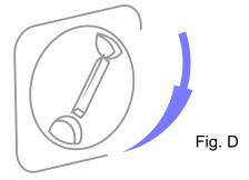
The drain filter protects the pump from lint and foreign matter and MUST be cleaned regularly.
